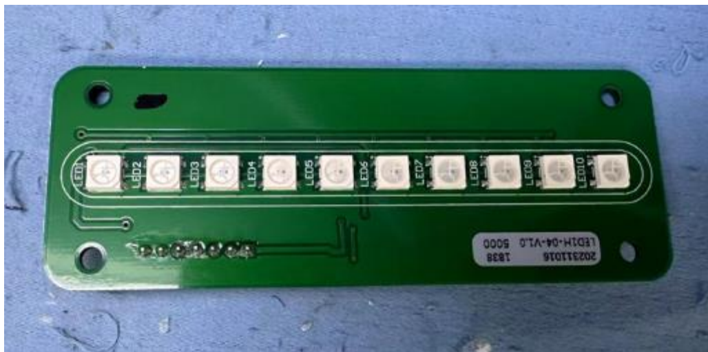
Photo 21 - LED PCB view of PEV-40A09US, PEV-48A09US, PEV-40A09NACS and PEV-48A09NACS
