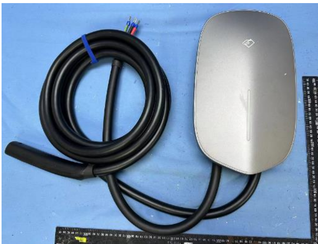
Photo 18 - External view of PEV-40A09NACS and PEV-48A09NACS
