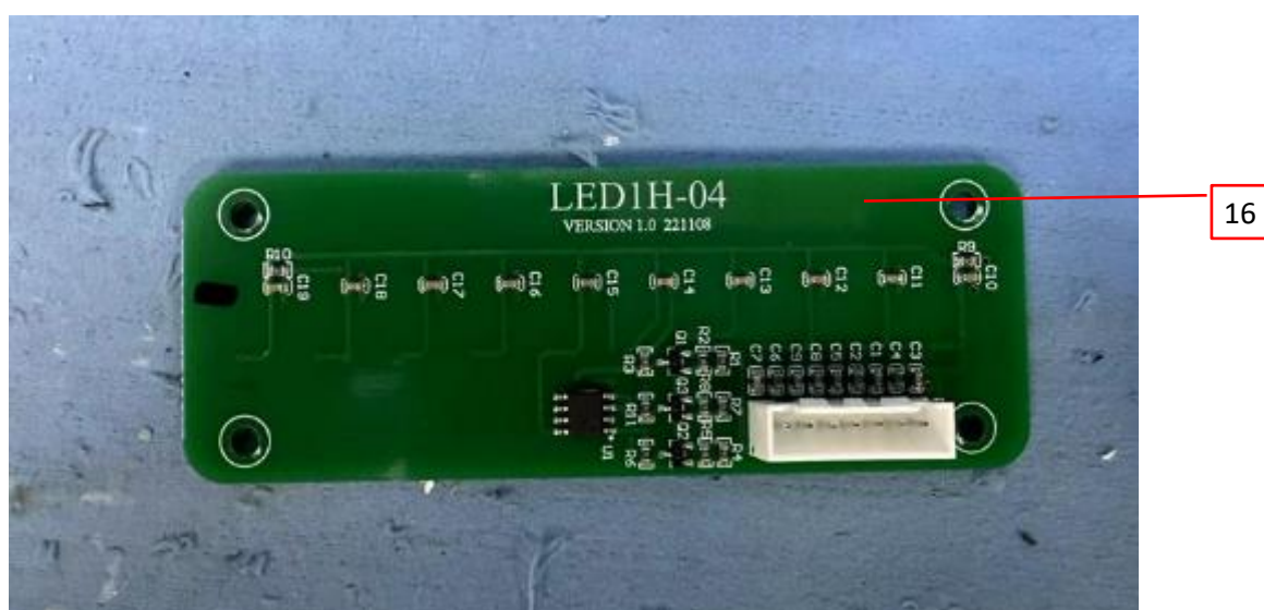
Photo 20 - LED PCB view of PEV-40A09US, PEV-48A09US, PEV-40A09NACS and PEV-48A09NACS
